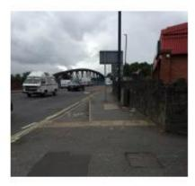
38. Bath Road west side – road sign posts in the roadway at the cycle slip road, pictured above, create an obstruction: space between the posts is 88cm and between the right-hand post and the kerb is 110cm
